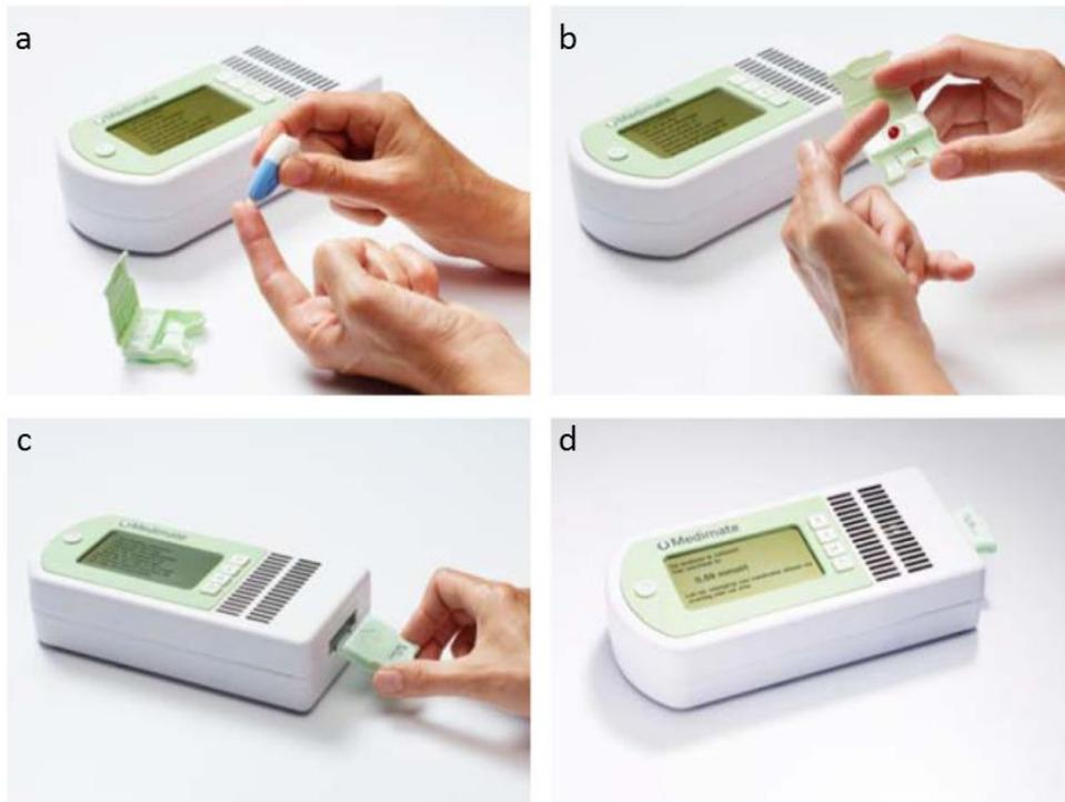
Figure 2: Performing a measurement on the Medimate Minilab®. A finger stick is performed with the finger stick pen (a), after which the blood droplet from the finger is applied to the Lab-chip (b). Then the Lab-chip is inserted into the Multireader (c) and finally after a few minutes the concentration value is shown on the screen (d).
