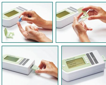
Figure 1: Measurement steps. 1. Perform fingerstick, 2. Apply blood droplet, 3. Insert Cartridge, 4. Readout result
