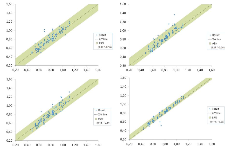
Figure 2: Patient (top left), physician officer (top right) and specialist (bottom left) Medimate Minilab fingerstick measurements are compared by Method Comparison with fingerstick plasma measurements on the IL943 reference method. The shaded area encloses 95% of the measurements. Bottom right serum results performed by the specialist. X-Axis lithium [mmol/l] IL943 reference method. Y-Axis lithium [mmol/l] Medimate Minilab.
