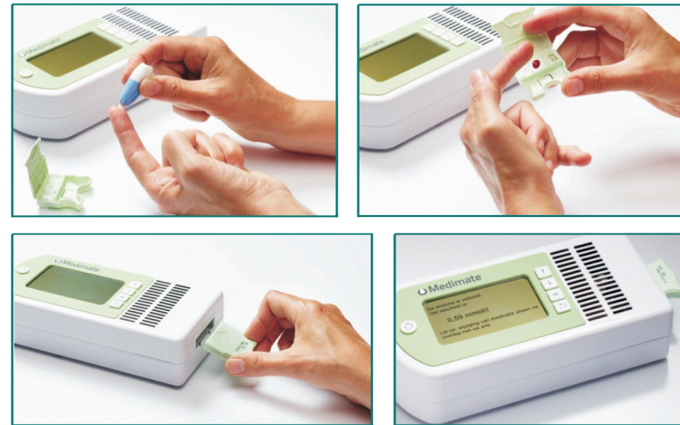
Figure 1: Photo of Medimate minilab measurement steps. 1. Perform fingerstick, 2. Apply blood droplet, 3. Insert Cartridge, 4. Readout result
